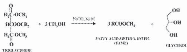
Scheme 1. Transesterification reaction of vegetable oils to produce FAME (biodiesel) and glycerol as by-product.
